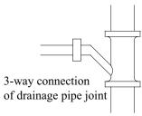
NO2: Connection of drain elbow
