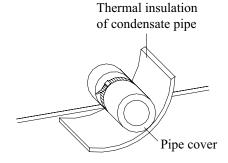
6.2.15 The long drainage pipe may be fixed by using hanger bolts, thus to ensure a gradient of 1/100 (PVC cannot be bent).
