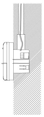
Fig.6.5.5 Concealed Cable Installation 2 (up-down wiring)
