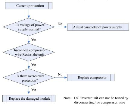
Overcurrent occurs in operation, i.e. the indicator will display the current protection just after startup.
