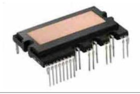
The PFC module integrates 4 diode tubes and 2 MOS tubes. They convert the AC input power into DC power. Meanwhile, the connection and disconnection of MOS tube is controlled via PWM wave, thus to realize the voltage rise under the function of electric induction.
