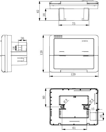
Fig.6.5.1 Installation Dimensions Diagram
