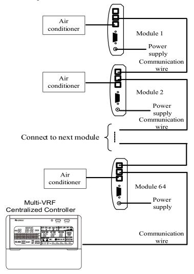
Fig.7.2.6.1 Skecth map of connection between centralized controller and communication module
