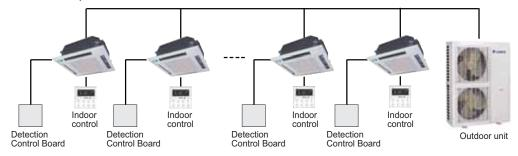
Fig.1 Communication Network of Detection Control Board for GMV series
