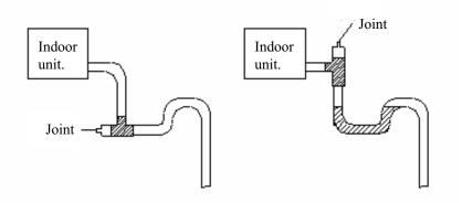
6.2.17 Connection of drainage branch pipe to the standpipe or horizontal pipe of drainage main pipe.
