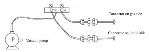
Start the vacuum pump and turn on "LO" and "HI" knobs;
