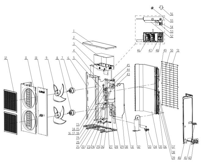
GMV-Pd140W/NaB-M for CN850W0032,GMV-Pd160W/NaB-M for CN850W0140,Part List
