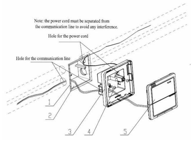
Fig. 6.5.6 Installation Diagram
