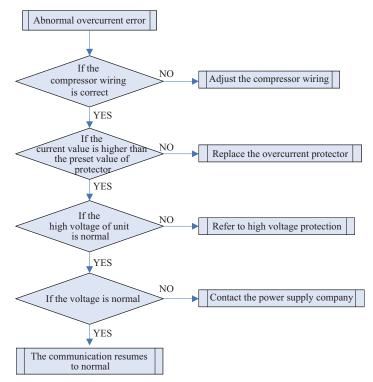
Upon AC inverter startup overcurrent, the indicator will display the current protection.
