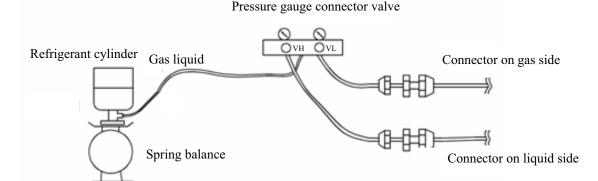
b. Open pressure gauge valve VH, then fill liquid state refrigerant into the liquid pipe side until required amount is reached.
