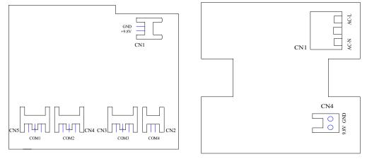
Fig.6.5.2 Interfaces of the Display Board
