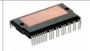
The IPM module integrates 3 pairs of complementary IGBT tube and controls their connection and disconnection via PWM wave, so that the DC bus voltage is applied to different stator windings of the compressor in different time section and the current is hence generated on the stator. Meanwhile, magnetic field is induced on the rotor windings, thus to push the rotor and drive the compressor to run.
