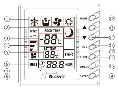
Fig.4.1.1.1 Wired Controller Z60351F,Z60151F
