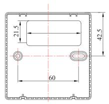
Fig.4.1.2.2 Installation Dimension of Wired Controller
