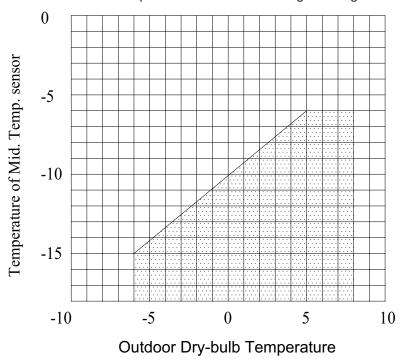
Or the outdoor ambient temperature is below -6°C; and keeps heating (the four-way valve is under the heating position) for 2 hours;
