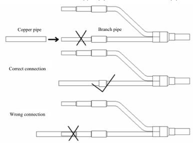
The copper pipe shall not be inserted into the branch pipe too deep.
