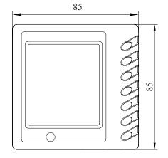
Fig.4.1.2.1 Outline Dimension of Wired Controller
