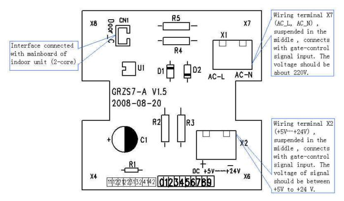
Fig2: Detection Control Board Interface Sketch
