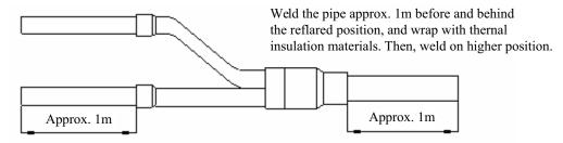
i. To avoid the position difficult to weld, you may add a prefabricated assembly below.
