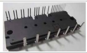
PFC module It used for GMV-Pd100W/NaB-K, GMV-Pd120W/NaB-K, GMV-Pd140W/NaB-K, GMV-Pd160W/NaB-K,
